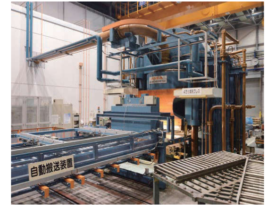
40,000 ton press, one of the largest in the world
