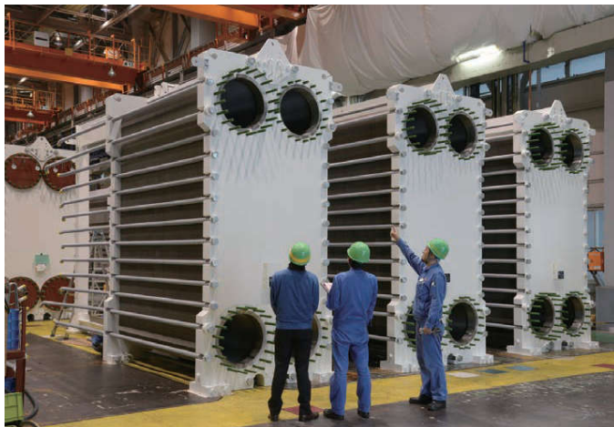
UX-160, one of the largest plate heat exchangers in the world
