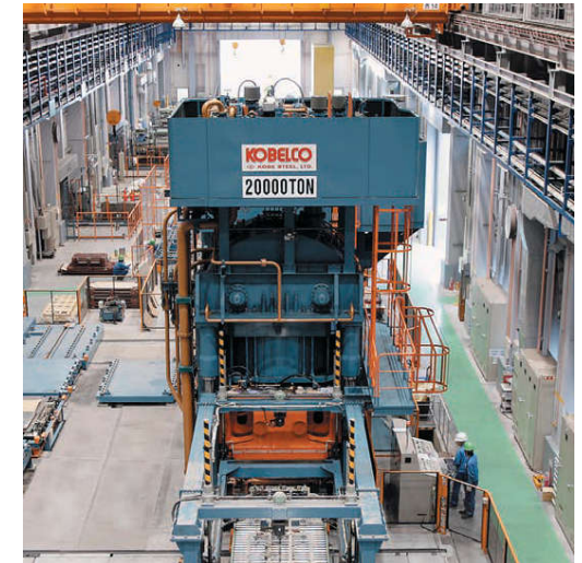
Fully-automated 20,000 ton press
